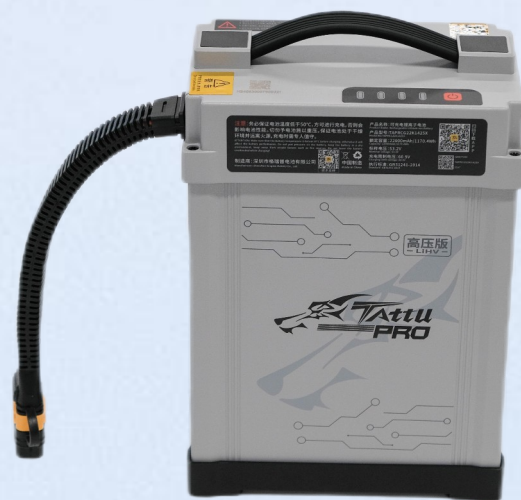
Smart battery 14S 22000mAh *1
