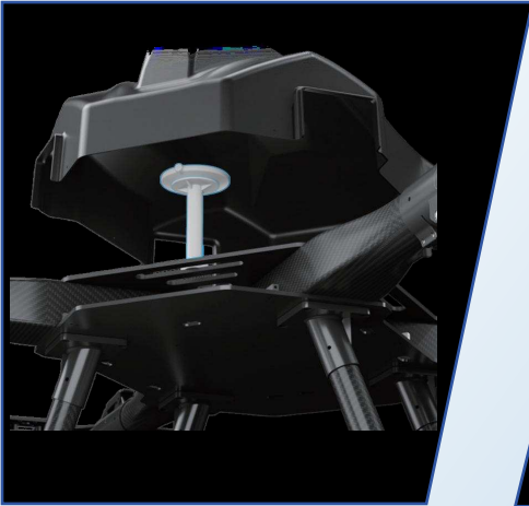
GPS Installation Position
